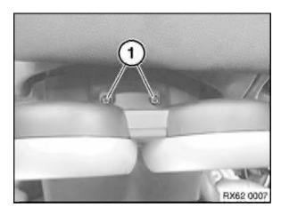
Release screws (1) on rear side of instrument.
