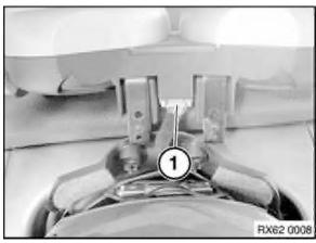
Unlock plug connection (1), disconnect and remove instrument.
